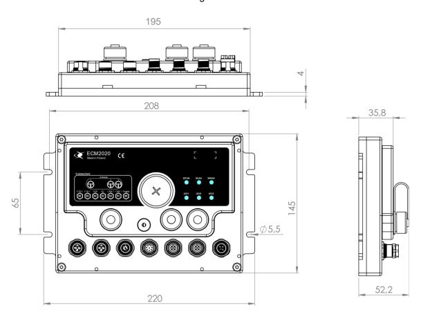
The preferred mounting position is connectors pointing downwards. If the unit is mounted connectors pointing to the side, then it is vital to leave some loose cable with a downward cue to prevent the ingress of moisture through connector.
